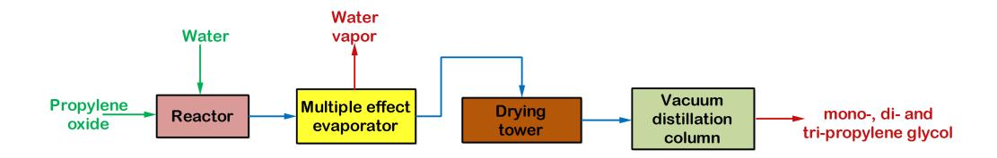
Figure: Manufacture of propylene glycol by hydrolysis of propylene oxide
